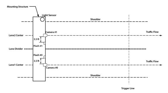
Figure 6. Typical Over Lane Site Layout Plan
